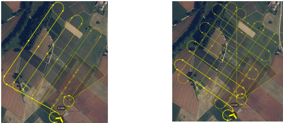
Figure 4. Traditional orthogonal flight plan and 2 perpendicular directions flight plan on quite a homogenous surface.
