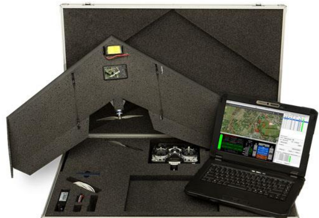
Figure 1. Swinglet CAM (© senseFly Ltd.)
