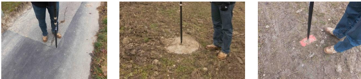
Figure 5. Examples of GCP (artificial and natural).
