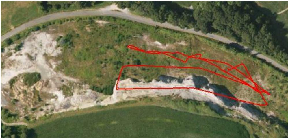
Figure 4: UAV flight: first programmed with a nadir position camera, then manually with an oblique view
