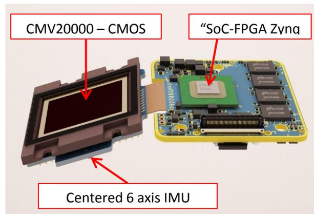
Figure 3: the CMOS Sensor with the inertial sensors and the embedded intelligence
