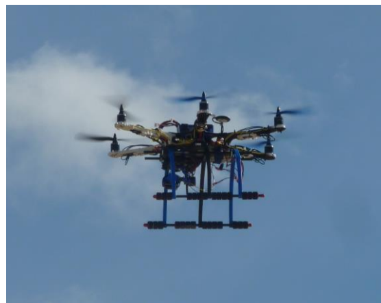
Figure 2: The UAV used during the flights, based on a modify F550 DJI frame.
