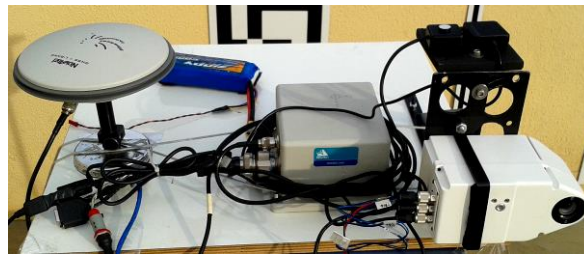
Figure 3: The RIKOLA DT camera mounted on a terrestrial platform.
